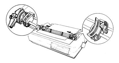
6. Fit the holes of the paper over the tractor pins of the sprocket units, adjusting the position of the sprocket units as necessary.
